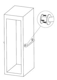
The left/right handle and fixing screw are packed inside the compartment. Take out and screw in the side handles before use.
