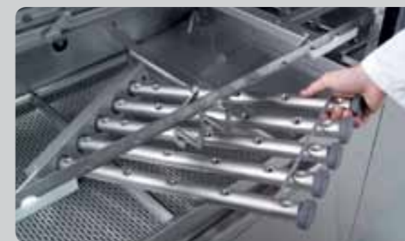
Easy to remove washing arms for quick cleaning.
