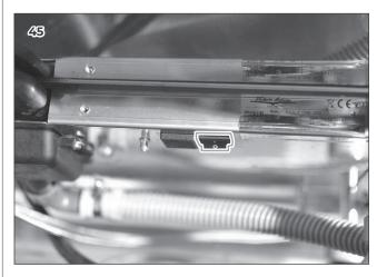
6 Push and stop after a few seconds a coffee dispensing button of the interesting infusion group, to partially empty the coffee boiler and reduce its inner pressure.
