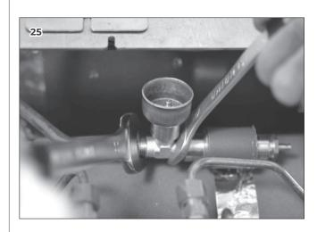
2 Utilizing a 17 mm wrench keep blocked the assembly and utilizing an adjustable clamp unscrew the valve.
