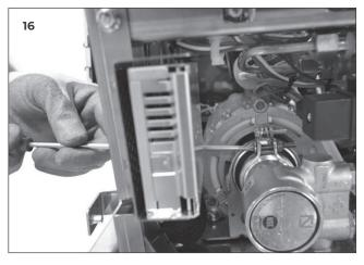
8 Utilizing a 21 mm wrench and a 17 mm one, unscrew the unions and adapt them to the new pump utilising Teflon tape to seal the part.
