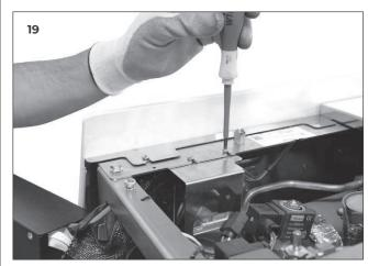
4 Remove the metal plate with the contactor.
