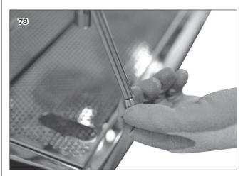
4 Utilizing a 9 mm wrench, block the upper part of the wand and, by hand, unscrew the middle part of the nozzle.
