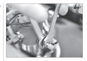
9 Utilizing a 13 mm wrench, remove the water input copper pipe.
