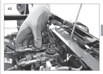
7 Utilizing a 7 mm wrench, remove the two screws fixing the flowmeter to the plate.
