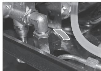
3 On the lower side of the coffee boiler, disconnect the heating element.
