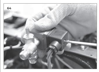
Since the cold water valve is connected with a tap, it may be necessary to replace the whole part.
