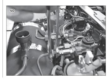
5 Utilizing two 17 mm wrenches, remove the incoming copper pipes from all flowmeters.
