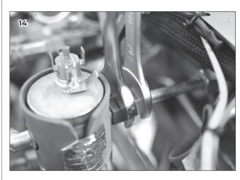
11 Take off the boiler paying attention to water spilling.
