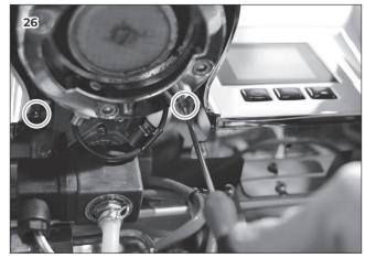
3 Rotate the group cover from the top downwards to remove it from the machine.
