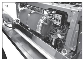
3 Utilizing a Philips screwdriver, loosen the three screws on the bottom.
