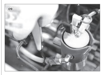
6 Disconnect the exhaust pipe of the expansion valve.
