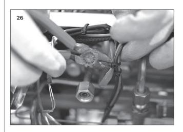
4 Following the orange cable, disconnect the heating element from the neutral and from the high-limit thermostat.
