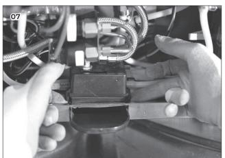
4 Utilizing a 17 mm wrench, unscrew the bolt inside the drain box.
