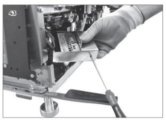
4 Utilizing a Philips screwdriver, disconnect all cables.
