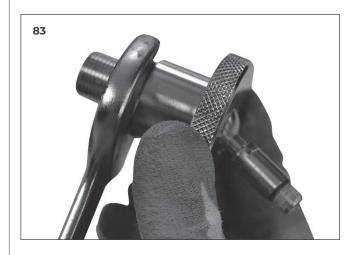
9 The junction is visible now, with its spring. Notice that there is a white Teflon o-ring inside the joint.
