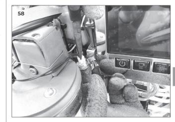
3 Utilizing a small flat screwdriver, press the three little wings and push down the led.
