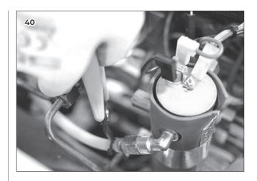
4 Disconnect the exhaust pipe of the expansion valve.
