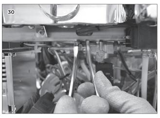
8 Utilizing a Philips screwdriver, from the top of the machine remove the screw fixing the auto-fill valve to the frame.
