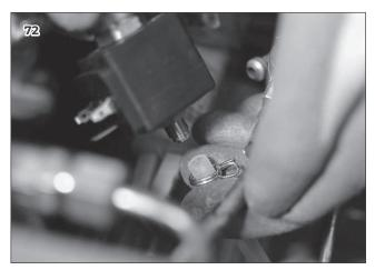
10 Utilizing a 14 mm wrench, unscrew the nut and remove the coil of the valve.
