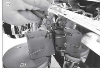
4 Utilizing a 13 mm wrench, loosen the sensor fixing nut.
