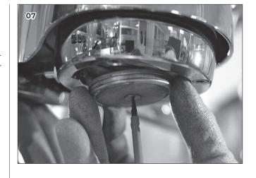
To change the seal use an awl or a slim flathead screwdriver and at first remove one edge of the seal and then remove it entirely. If the group is worn out just insert shims under the seal so as to reduce the stroke of the filter holder.
