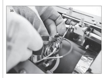
4 Utilizing a 3 mm Allen Key, remove the screw holding the probe to the group.
