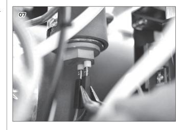
4 On the higher side, disconnect the ground and the high-limit thermostat.
