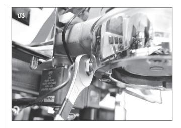
5 Utilizing an adjustable wrench, slide out the sensor.
