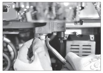
5 Disconnect the Teflon pipe of the third outlet.
