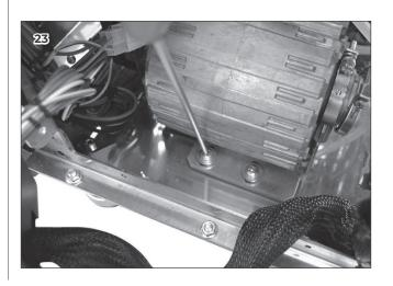
6 Carefully remove the motor from the left side and disconnect power connections.
