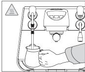
By pulling it completely the lever will hold a position of maximum delivery; by pushing it, the lever will automatically give way.
