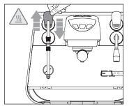
Before use the steam wand, cleaning out of the condensation for at least 2 seconds.
