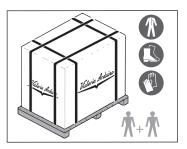
The machine is transported on pallets containing several machines inside cartons strapped to the pallet.
