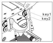
set the second hot water 6 To confirm and exit, press serving size (key 2).
