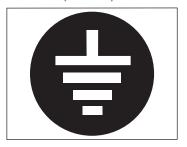
The manufacturer cannot be held responsible for any damages incurred if the system is not grounded. For electrical safety, this machine requires a ground system. Contact a technically certified electrician who must check that the line electrical capacity is adequate for the maximum capacity indicated on the machine label.
