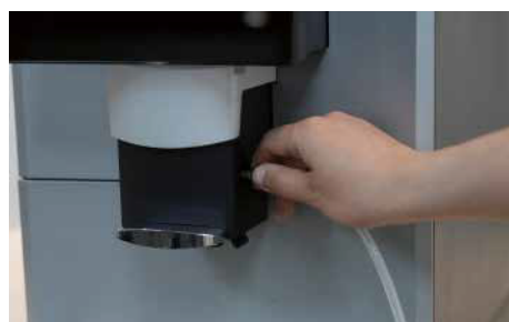
1. Connect milk pipe to machine
