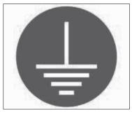
For electrical safety, this machine requires a ground system. Contact a technically certified electrician who must check that the line electrical capacity is adequate for the maximum capacity indicated on the machine label.
