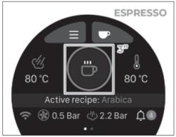
If the machine is in PureBrew brewing mode, select Espresso mode by pressing the centre icon for 3 seconds.
