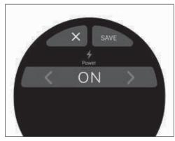
to ac- From the **Technical Settings** menu, press to access the Power Management func-Offset indicates the difference from a meas- tion, which allows you to limit the power consumption of the machine. Temperature probes may be slightly different Enable (ON) or disable (OFF) the consump-
