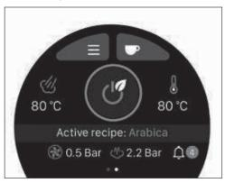
Press the icon for 3 seconds to turn the machine to **Standby**.
