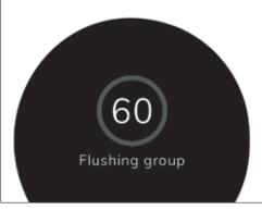
The countdown for the rinsing phase is visible on the display.
