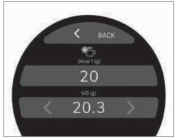
Press on the set value to access the VIS calibration.
