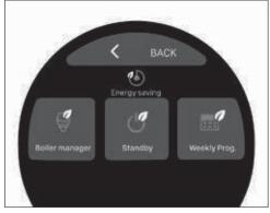
You can optimise the power consumption of the machine according to your needs, by enabling (**ON**) or disabling (**OFF**) the coffee dispensing unit and/or the steam nozzle.
