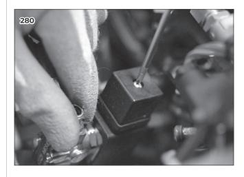
Use pliers, remove the clip and the Teflon pipe of the third outlet.
