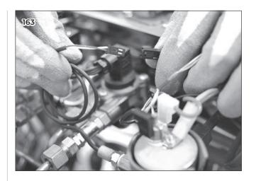
Use a 12 mm wrench and a 13 mm to remove the temperature probe.
