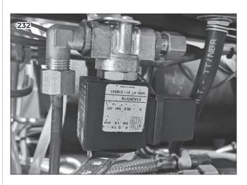
Use a Philips screwdriver unscrew and remove the head of the auto-fill valve.
