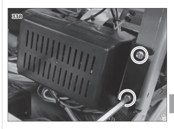
Use a 7 mm wrench, remove the two screws holding the plate.
