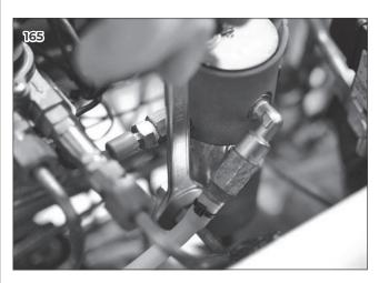
Use two 17 mm wrenches, remove the water output copper pipe.
