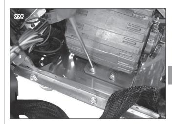
Carefully remove the motor from the left side and disconnect power connections.
