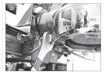
Use an adjustable wrench, slide out the sensor.
