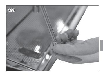
Use a 9 mm wrench, block the upper part of the wand and, by hand, unscrew the middle part of the nozzle.
