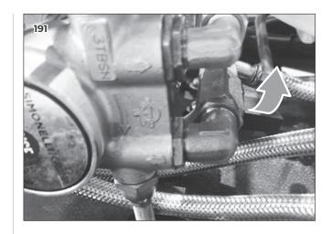
Cut the clamp of the exhaust pipe of the expansion valve.
