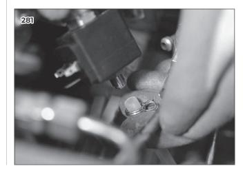
Use pliers, remove the clip to remove the coil.
