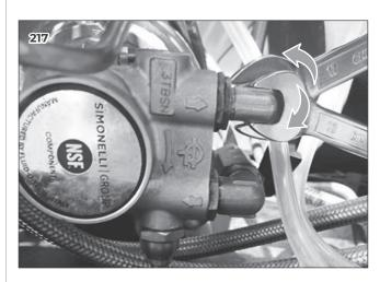
Unscrew the metal hose clamp that keeps the pump attached to the motor and remove it.
