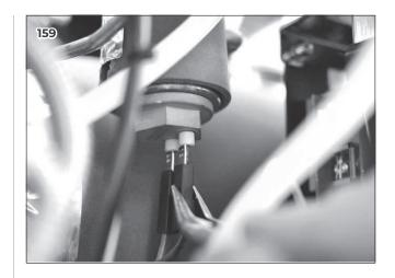
On the higher side, disconnect the ground and the high-limit thermostat.
