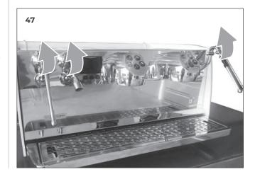
Remove the work surface raising and removing the water collection pan.
