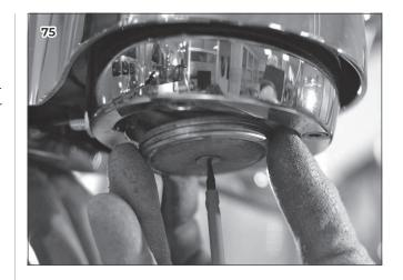
To change the seal use an awl or a slim flathead screwdriver and at first remove one edge of the seal and then remove it entirely.
