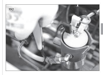
Disconnect the exhaust pipe of the expansion valve.
