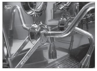
Use a 24 mm wrench **A** and a 20 mm wrench **B**, block the front fitting and unscrew the copper pipe.
