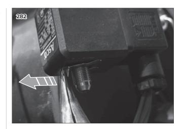
Use a bench vise and a 22 mm wrench, unscrew the valve base.
