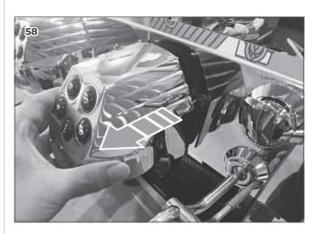
Rotate the group cover from the top downwards to remove it from the machine. If necessary, disconnect any connections.
