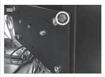
Unplug the connector **A** by hand and all the cables with the help of a Phillips screwdriver.
