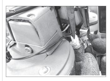
Use a small flat screwdriver, press the three little wings and push down the led.
