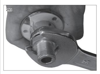
The junction is visible now, with its spring. Notice that there is a white Teflon O-ring inside the joint.
