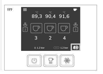
If the error indicates a coffee boiler temperature probe issue, possible solutions are:
